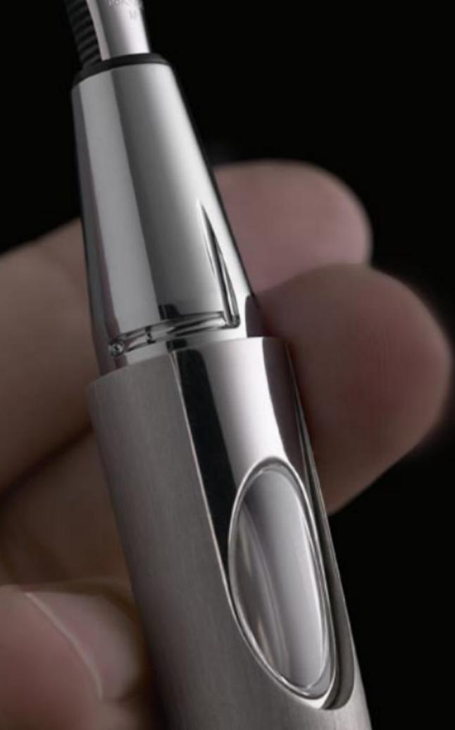
*To ensure the perfect closure of the cap, and a precise line-up of the different parts, an unusual and advanced bayonet system has been created, made possible by using a stainless steel micro-sphere, which is inserted in the cap within an elastic ring system which allows its breathing while the ball runs along the mill-made groove on the steel nib grip up to the point where it secures the cap with a soft click.*
